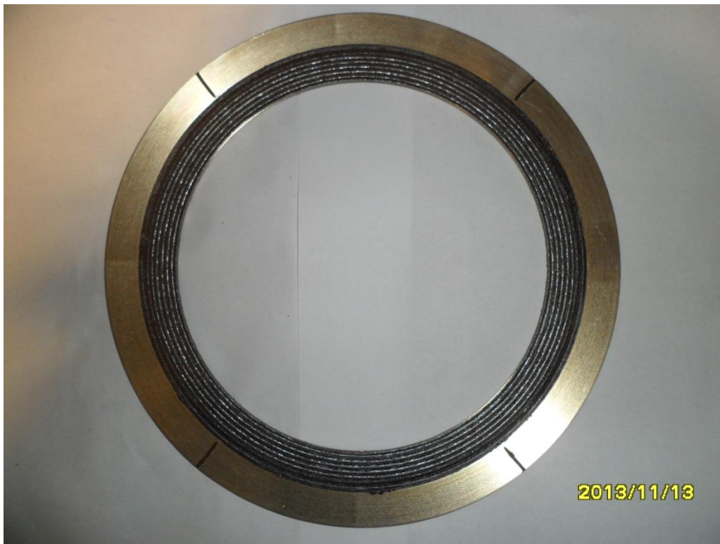
Grooves cut in out ring to prevent sealing.
