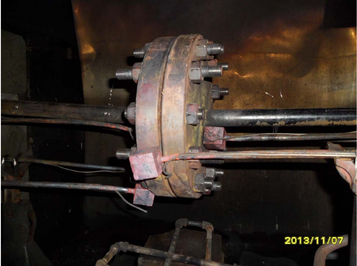
Test Gasket Setup Prior to Burn
